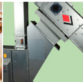
Connection hopper between conveyor and elevator.
