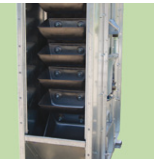
Antistatic bucket belt with steel buckets.
