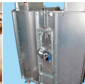
Belt tension in boot & speed monitor.
