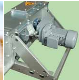
Direct-mounted gearbox motor with support frame.
