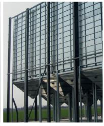
**STORAGE BINS TYPE ST** Tornum Type ST square bins come with a 45° hopper in a wide range of sizes.
