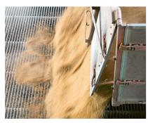
**RECEIVING PITS** Tornum receiving pits are available in different sizes and are delivered complete with run-over rails. Our receiving pits are designed to be connected directly to the conveyor.
