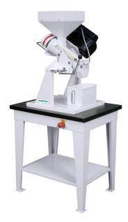
The LA-P small-scale de-awner is designed for batch operation; the main purpose of de-awning is to remove awns from barley kernels, loose husks from wheat, etc. However, this machine is not suitable for very small seeds.
