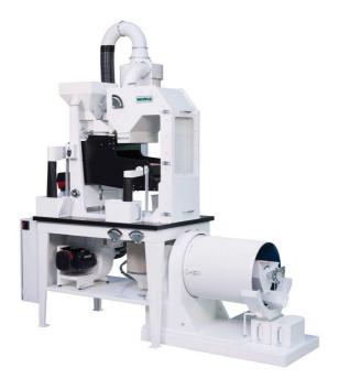
The LA-LST small-scale air/screen cleaner with integrated indented cylinder is a precision and fine cleaner/grader for research stations, institutes etc.
